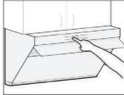
4. Hold the two sides of the grease filter and pull sideward to unlock it.
