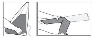
7. Lift and position the hood onto the mounting screws. Make sure the hood is stable and leveled by using a spirit level. Install the safety buffer baffle above the hood.
