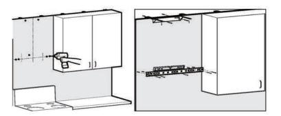
Caution: One of the screws for duct bracket must be fastened to the wooden beam.
