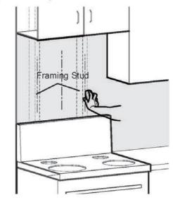
3. Locate the duct bracket. Determine the central point and mark the centerline on the wall where the hood will be installed. Also, mark the point where the central line and the lowest point on the bottom board of the top cabinet meet. This is the location, in which to secure the bracket. Mark screw hole locations on the wall. The distance between the lowest point on bottom board of the top cabinet and the center of the bracket should be 16" (405mm).
