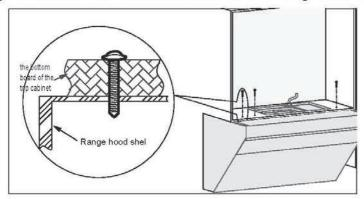
of the top cabinet and the top of the range hood, please add wood pads based on the gap size near the three M5×70 screws to avoid range hood shell deformation caused by the tightening of screws, which will affect the use of the range hood.
