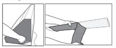
7. Lift and position the hood onto the brackets at the bottom of the backside while keeping an angle between the wall and the hood, and then push the hood against the wall tightly.
