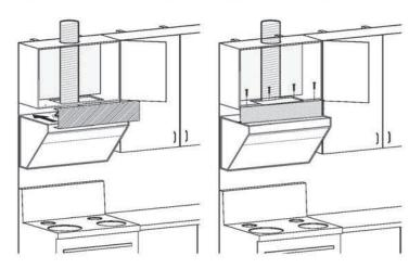
10. Make sure the hood is leveled. Install the Grease Cup, and plug the appliance for a test run.
