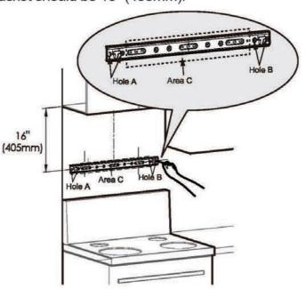
4. Fasten the bracket: drill  $\phi 3/8$ " ( $\phi 8$ ) hole at the screw hole marks with electric drill, embed expansion tubes and fasten the bracket with bracket screws. Use leveling instrument to make sure that the bracket is leveled.
