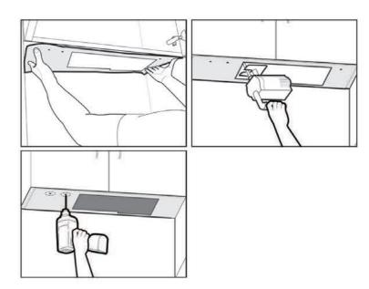
Caution: Wear safety goggles when drilling. In case of batten at the wall facing the bottom plate, the rear wall side of the paper template shall be cut as per the thickness of the batten.
