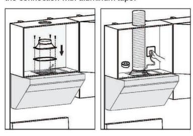
10. Make sure the hood is leveled. Install the Grease Cup, and plug in the appliance for a test run.
