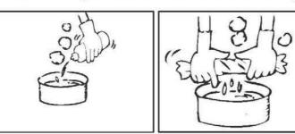
Washing and cleaning the surface, Grease Cup, and grease filter: (The cleaning can be done by the user)
