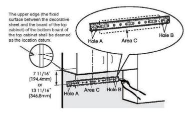
4.Fasten the bracket: drill Ø8 hole at the screw hole marks with electric drill, embed expansion tubes and fasten the bracket with bracket screws. Use leveling instrument to make sure that the bracket is leveled.
