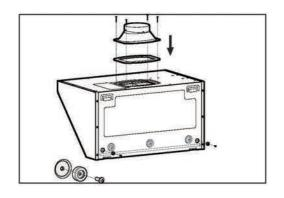
8. Lift and position the hood onto the brackets at the top of the backside while keeping an angle between the wall and the hood, and then push the hood against the wall tightly. Secure the duct to the duct cover and seal the connection with aluminum tape.
