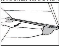
Warning: For the safety of you and your family, please regularly clean the oil accumulated in the Grease Cup and deposits on the Grease Cup surface. Do wear qualified protective gloves.
