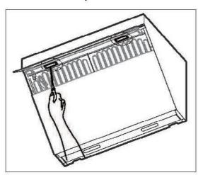
Disconnect the wires and then replace the LED lights.
